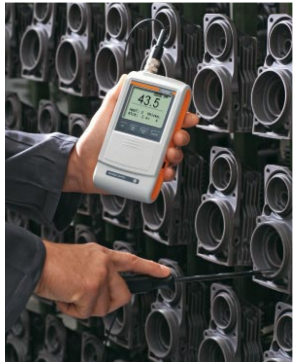
Measurements using the internal probe FAI 3.3-150
