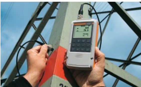
DUALSCOPE® FMP40 using the duplex probe FDX10 in outdoor applications
